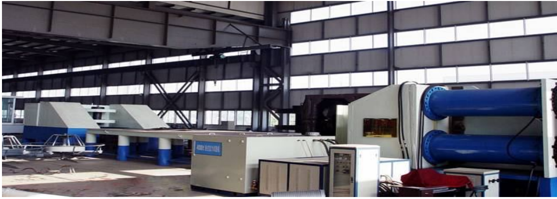
Breaking Load Testing of the whole tie rod system
