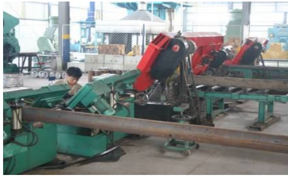
Materials Cutting: Preparing the materials for the tension rod, bearing plates, nuts, turnbuckles.etc
