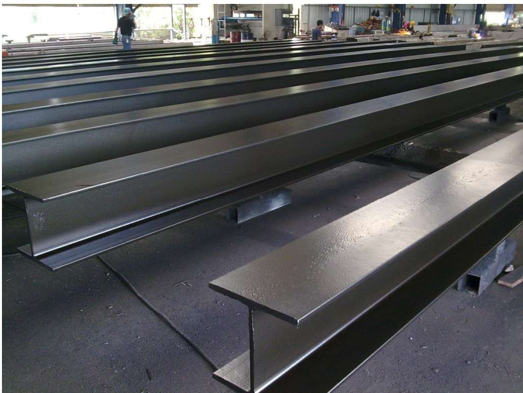
Hot Rolled H beams being painted in our works
