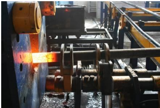
Upset Ends Forging for the tie rod shank, so that threads can be made on
