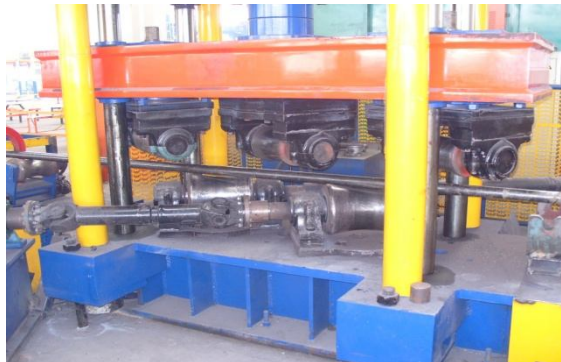
Adjust Bending of tie rod shank and Machinery of anchor
