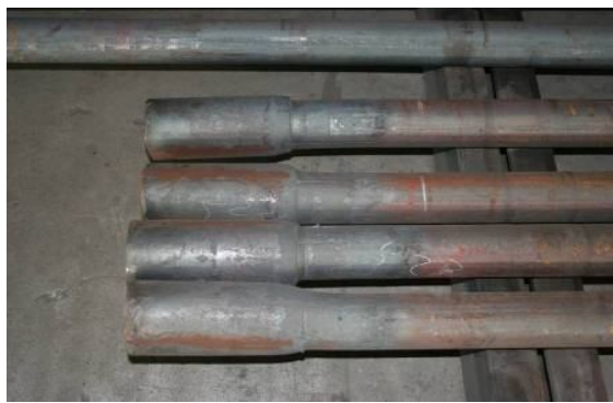
Upset Ends Forging for the tie rod shank, so that threads can be made on
