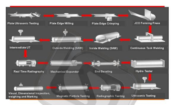
Production Process of LSAW pipes
