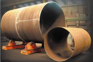
2m pipe segments welded together(big diameter)
